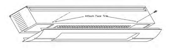
Optional Face Trim can be easily installed on all Sunpak models.
