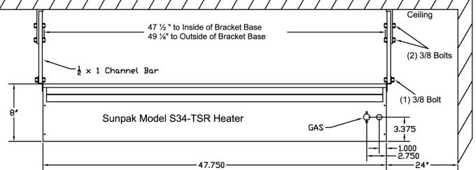
Warning: Heater must be level in the lengthwise direction.
