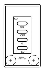
Two #2032 Button Batteries power the wall control transmitter They are available at your local hardware store.
