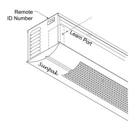
The Sunpak S34-TSR should <u>always</u> be started up and operated on the HIGH mode for the first 5 minutes to allow the heater to warm up. Starting up the heater on the LOW mode before the heater is warmed up may cause the heater to shut down prematurely. To correct this situation press the OFF button followed by the ON button and the HI button. Always PRESS the button for at least 1 second to allow proper transmission of the remote signal.
